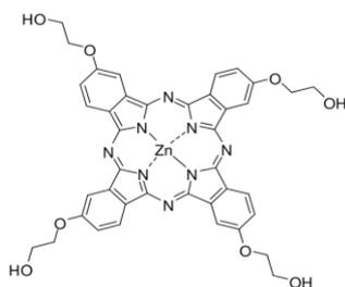
**Figure 1.** Phthalocyanine structure of ZnPcOH.
