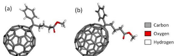
**Figure 3** – PC60BM (a) and PC70BM (b) structures.
