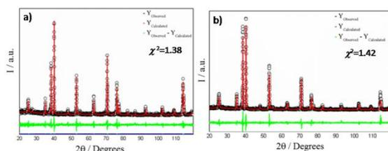
**Figure 1.** Rietveld refinement for a) TiO<sub>2</sub>NT-PTT and b) TiO<sub>2</sub>NT-LTT nanostructured materials.
