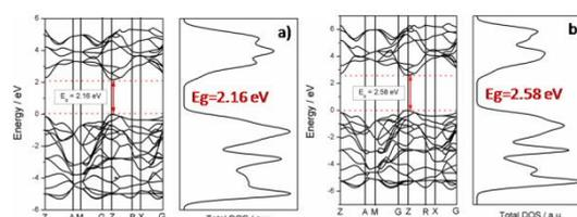
**Figure 2.** Band structure and DOS obtained for a) TiO<sub>2</sub>NT-PTT and b) TiO<sub>2</sub>NT-LTT nanostructured materials.
