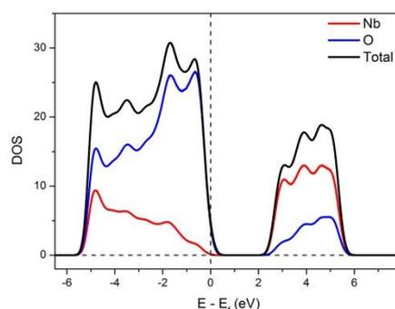
**Figure 1.** Total and projected DOS over the atoms of Nb<sub>2</sub>O<sub>5</sub>.
