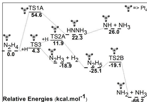
**Fig.1** Reaction profile for adsorbed molecules. Relative energies are given in kcal.mol<sup>-1</sup>.
