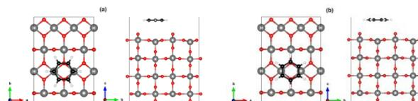
**Figure 1.** Optimized (a) benzene||TiO<sub>2</sub>-rutile and (b) benzene⊥TiO<sub>2</sub>-rutile.
