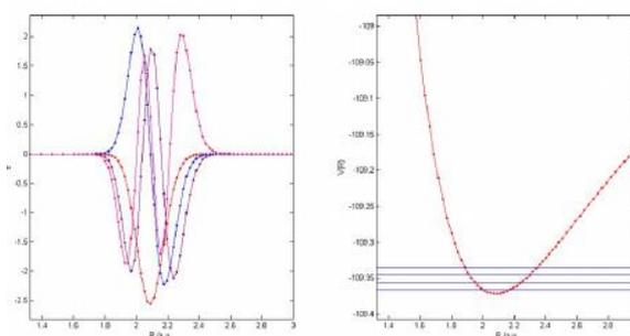
**Figure 1.** Anharmonic vibrational wave-functions (left) and their energy (right) for the first 4 states of N<sub>2</sub>.
