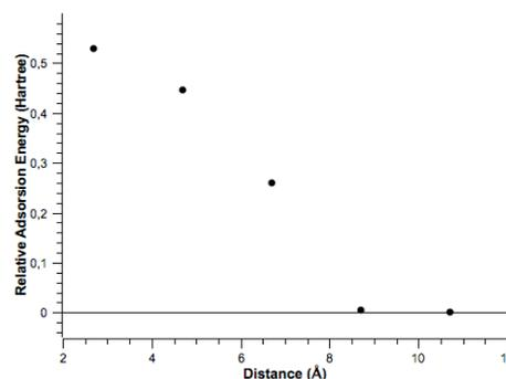
**Fig. 2:** Interaction energy dependence with the separation between pyrene and Pt cluster.
