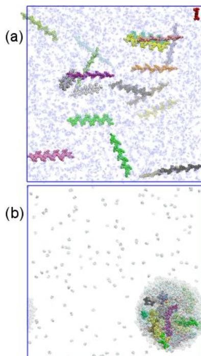
**Figure 2.** (a) Initial molecular system before the MD procedure. Box dimension with 25nm with
