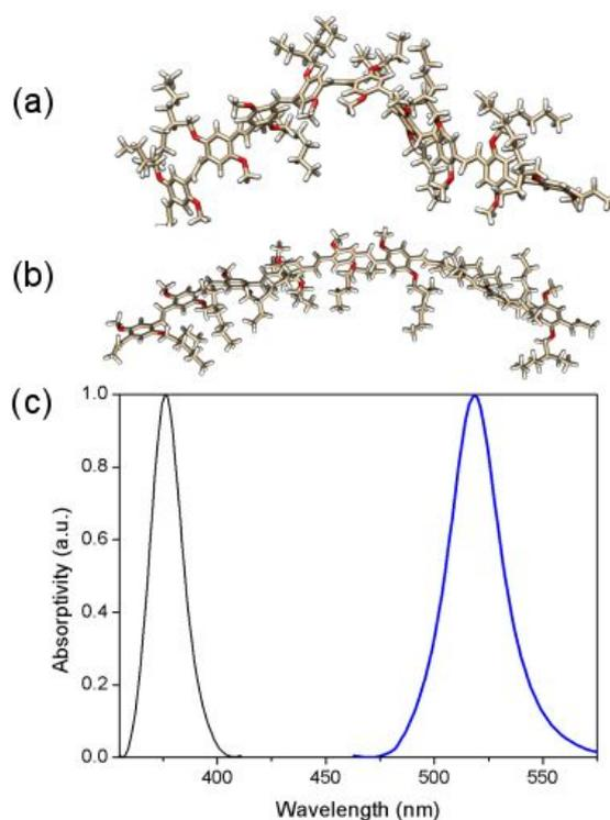
**Figure 3.** Conformational arrangements of two selected structures (a) twisted and (b) planar, from the sample after 5 ns of MD simulations. (c) Normalized first transition (HOMO-LUMO) from UV-Vis spectra calculated for these structures: in black color (for the twisted), and in blue color (for the planar); lorentzian broadening and a 11.28 half-width were added.
