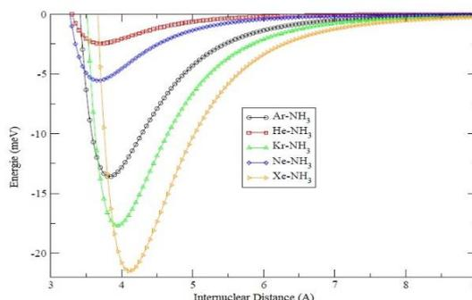
**Figure 1:** Potential energy curves for the interaction of ammonia with noble-gases.
