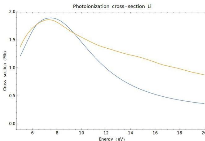
**Figure 1.** Photoionization cross-section of Li. In blue: our results. In yellow: experimental curve<sup>4</sup>.
