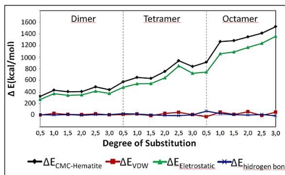
**Figure 3.** Binding Energy of CMC to Hematite.
